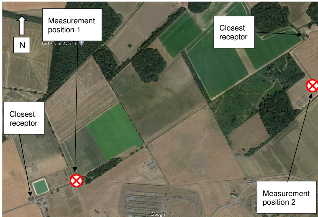
Figure 4 – Annotated aerial photograph of initial measurement positions © Google 2020
